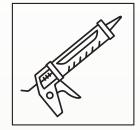
Caulking is used to seal gaps around corners, windows, doors and other exterior types of joints that can be exposed to water intrusion.
