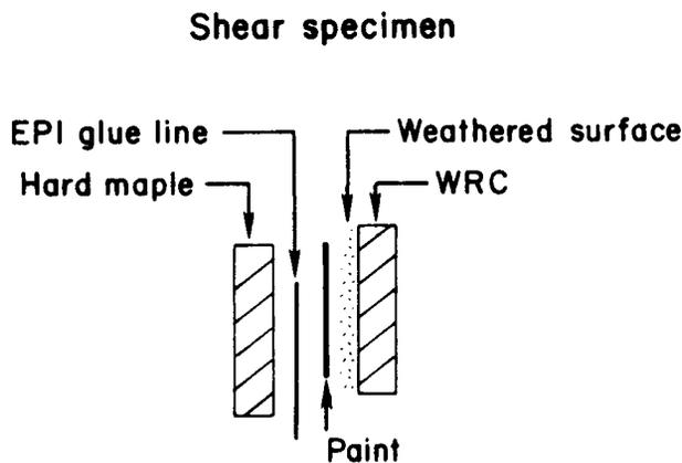
Figure 1. – Expanded drawing of block-shear specimen showing interfaces between the western redcedar (WRC) substrate and the maple panel.
