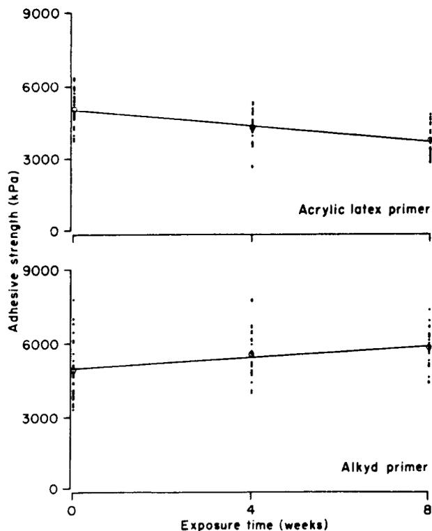
Figure 2. - Adhesive shear strength of Douglas-fir painted with acrylic latex or alkyd primer as a function of exposure time. Mean values are circles.
